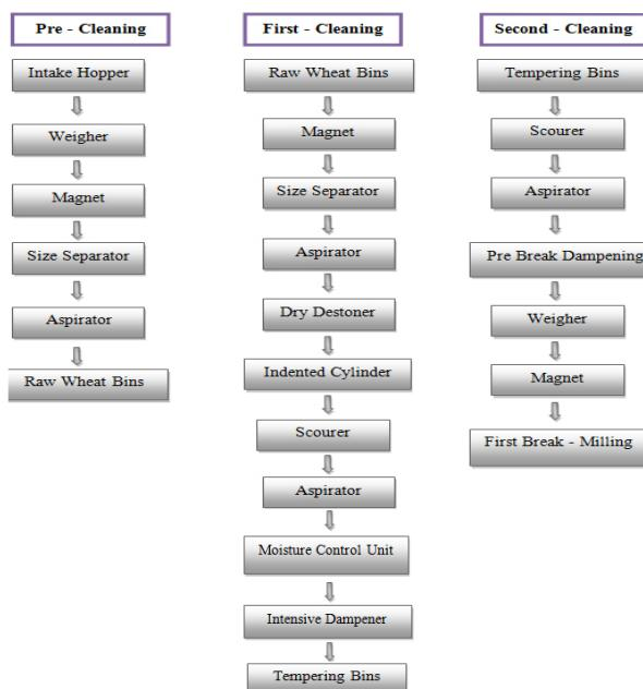
Figure 1. Basic flow diagram of typical wheat cleaning section prior to milling
