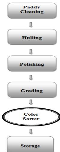
Figure 2. Optical sorting machine location in processing flow of rice milling
