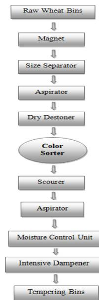
Figure 4. Integration of color sorter in first cleaning section: Location A.
