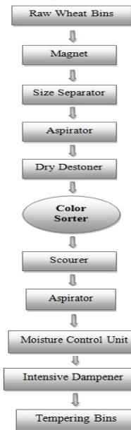
Figure 4. Integration of color sorter in first cleaning section: Location A.
