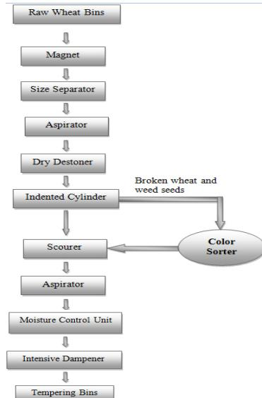
Figure 6. Integration of color sorter in first cleaning section: Location C
