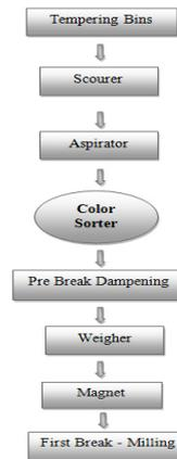
Figure 7. Integration of color sorter in second cleaning section
