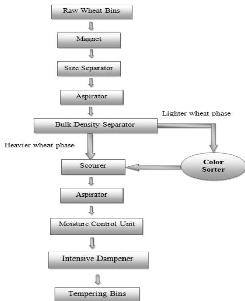
Figure 5. Integration of color sorter in first cleaning section: Location B.
