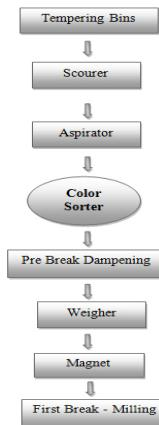
Figure 7. Integration of color sorter in second cleaning section
