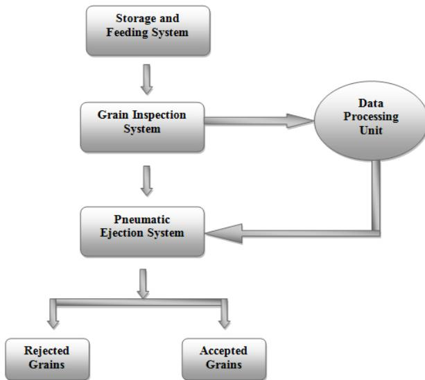
Figure 3. Schematic diagram of a typical optical sorting machine
